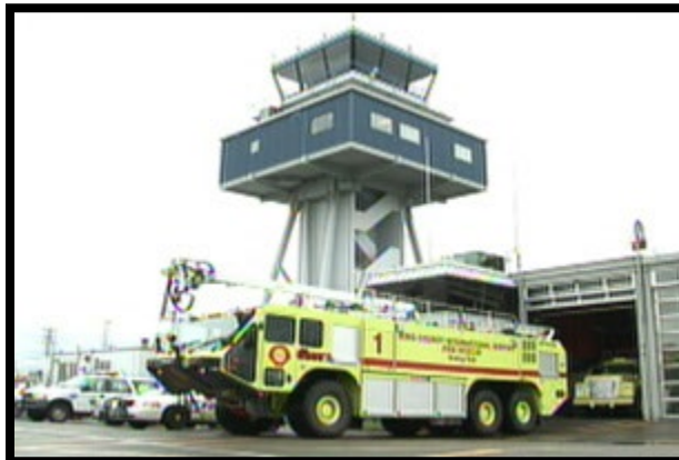
Oshkosh Striker - 3000 gallons of water with AFFF.
