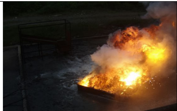
Prior to application of Novacool foam
