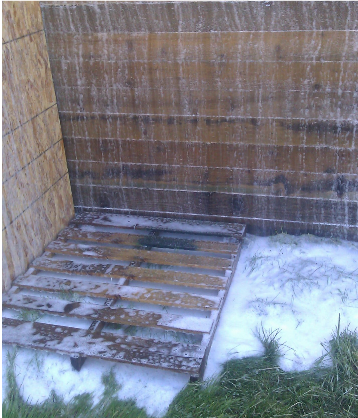
0.4% Novacool foam application, immediately after shutting down the nozzle
